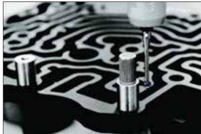
三次元測定機でねじ穴位置を測定 Measurement with three coordinate measuring machine
