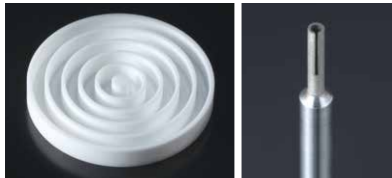
幅5mm深さ8mmの円弧溝加工 Processing arc grooves of 5mm in width 8mm in depth
